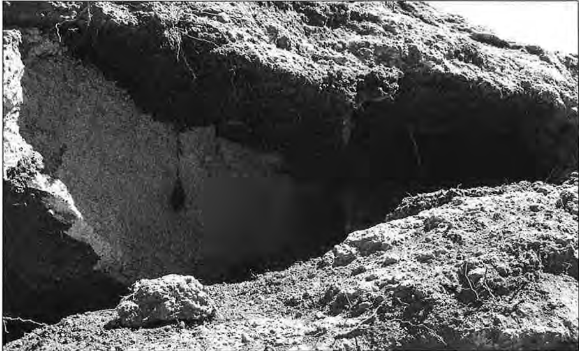
Figure 28 - Close-up of the break showing the internal faulting and separation.
